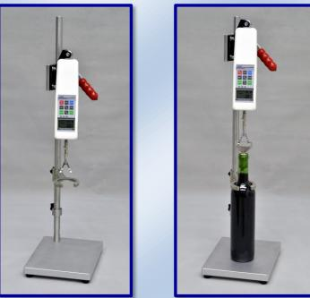
CET-1 Cork Extraction Tester is a force test system. It has been designed for wine producer and cork manufacturing industries. Easy to use, it allows to measure cork extraction or insertion and permits to improve the cork products and assembly/sealing process.
