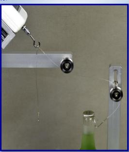
POT-1 has been studied and developed to be able to open step by step the pull off caps for carbonated beverages.
